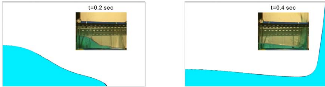
Figure 4 – Snapshots for the simulation instant 0.2 and 0.4 seconds compared with the experimental results presented by Koshizuka [1].
